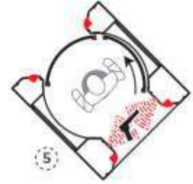
Person proceeds in. Upon disapproval from metal detector, system proceeds as programmed. (*)
